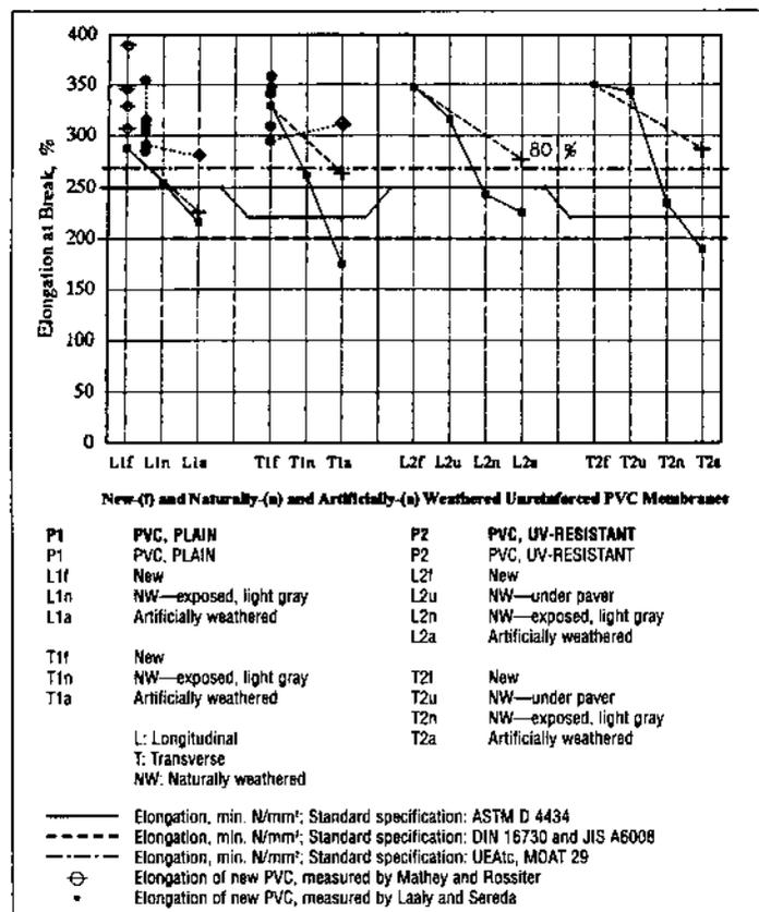
Figure 5. Comparison between longitudinal and transverse elongation of new (f), naturally (n) and artificially (a) weathered unreinforced PVC membranes and standard requirements.
