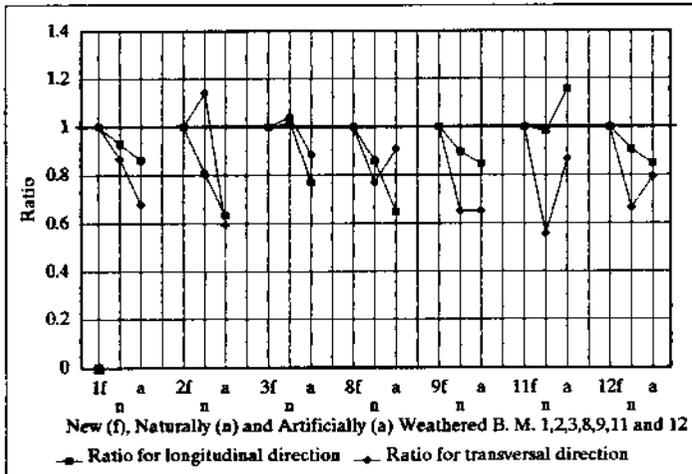
Figure 3. Ratio between longitudinal and transverse force x elongation of the naturally (n) and artificially (a) weathered APP modified bituminous membranes (B.M.) and force x elongation of the same but new (f) APP modified bituminous membranes.
