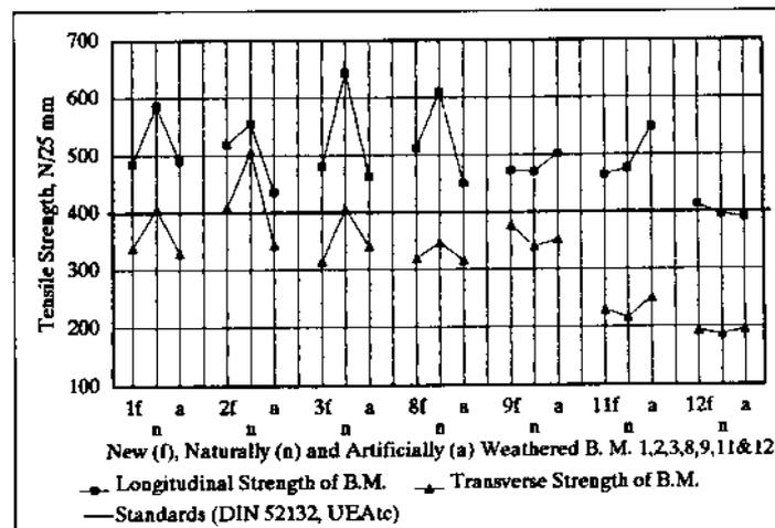
Figure 1. Longitudinal and transverse tensile strength of new (f), naturally (n) and artificially (a) weathered APP modified bituminous membranes (B.M.) and standards from DIN 52132 and UEAtc for comparison with.
