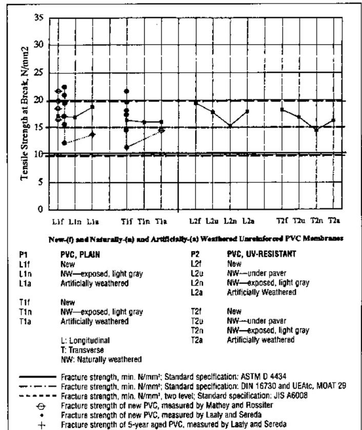
Figure 4. Comparison between longitudinal and transverse tensile strength of new (f), naturally (n) and artificially (a) weathered unreinforced PVC membranes and standard requirements.
