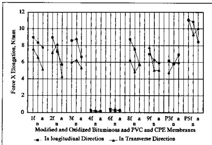
Figure 7. Longitudinal and transverse force x elongation of the new (f), naturally (n) and artificially (a) weathered modified and oxidized bituminous membranes and the new (f), naturally (n) and artificially (a) weathered PVC and CPE membranes.
