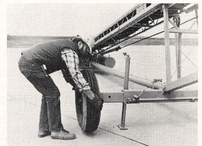
Built-in jacks take the weight off the wheels so telescoping axles can be pulled out.
