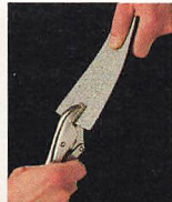
Pulling for Tensile Strength: No Failure.
