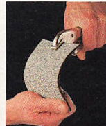
Bending at 0°F for Cold Flex: No Failure.
