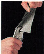
Twisting for Ambient Flex: No Failure.
