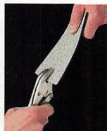
Pulling for Tensile Strength: No Failure.
