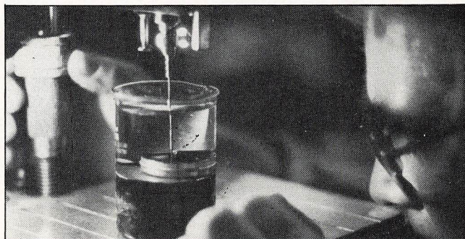
Lab Technician Dominic Serratore begins each penetration test by setting the test machine's needle precisely on the surface of the asphalt sample. To do this, he uses a bright light to create a reflection of the needle on the sample and adjusts the machine until the needle and its reflection just meet. Penetration is measured by the distance the weighted needle pushes into the sample during a five second interval.
