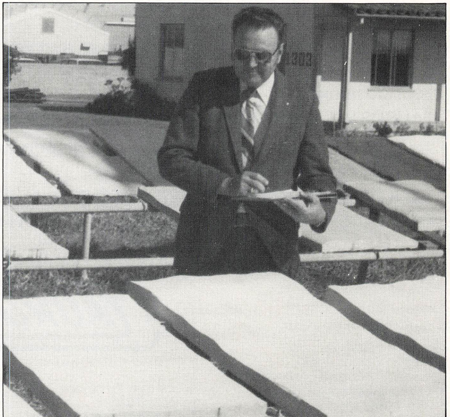
Robert Alumbaugh at the Naval Civil Engineering Laboratory checking the aging characteristics of various polyurethane roof tests.
