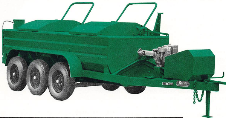
3 Axles-2 Covers-2 LP Burners w/Hi-Lo Controls
