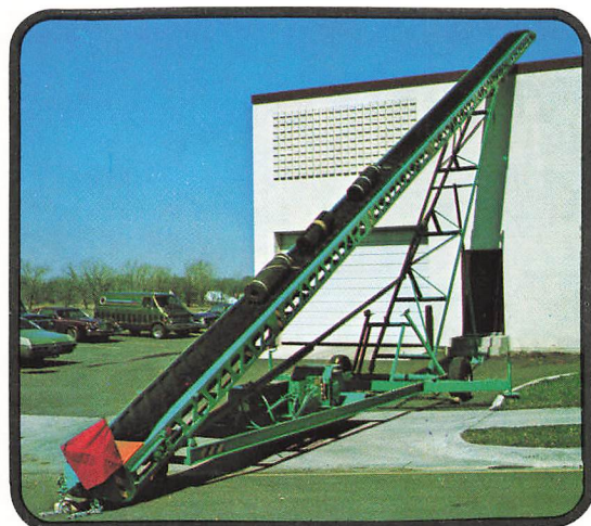
Handles rolls or insulation to high discharge height.
