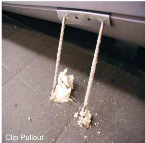
Failure of deck to joist connection
