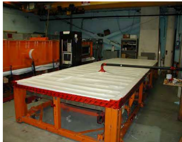
Figure 8: Installation of the impermeable cover
