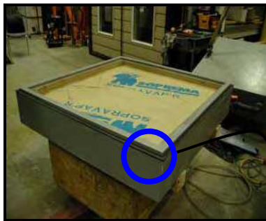
Assembly 3 – With Self Adhered Film (SAF) as air barrier material
