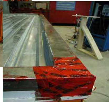
Figure 3: Deck Installation and edge treatment
