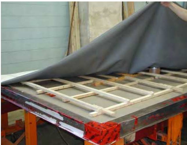
Figure 8: Installation of the impermeable cover
