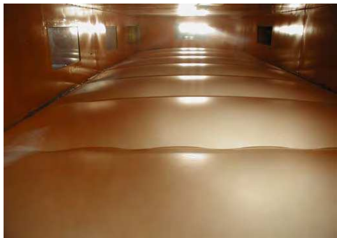
Figure 5: Response of mechanically attached membrane roofs under wind uplift testing
