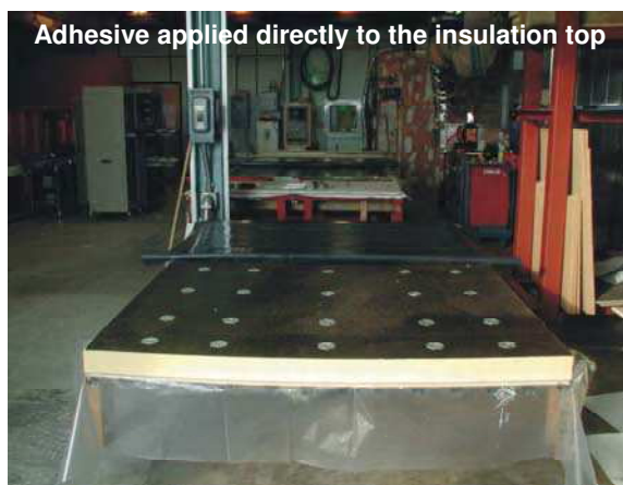
Figure 5. Mock up Construction Process of FBA with Barrier
