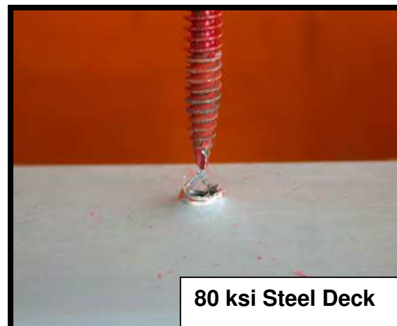
Figure 7: Experimental Setup for Fastener Pullout Measurements
