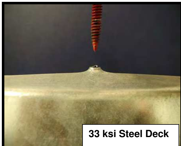
Figure 7: Experimental Setup for Fastener Pullout Measurements
