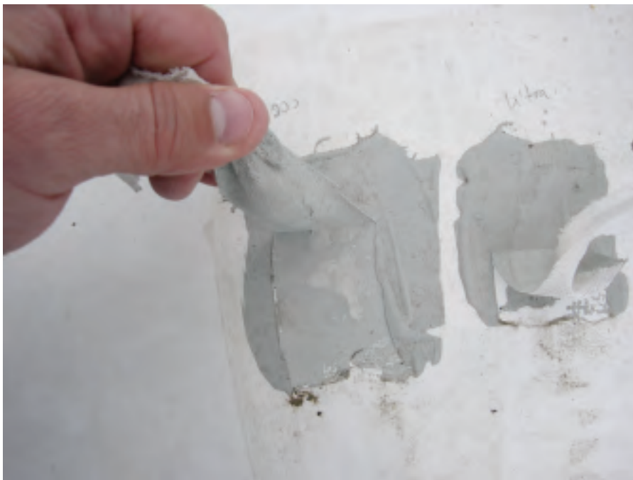
A field adhesion test, demonstrated in the photo, will help ensure a successful coating application.
