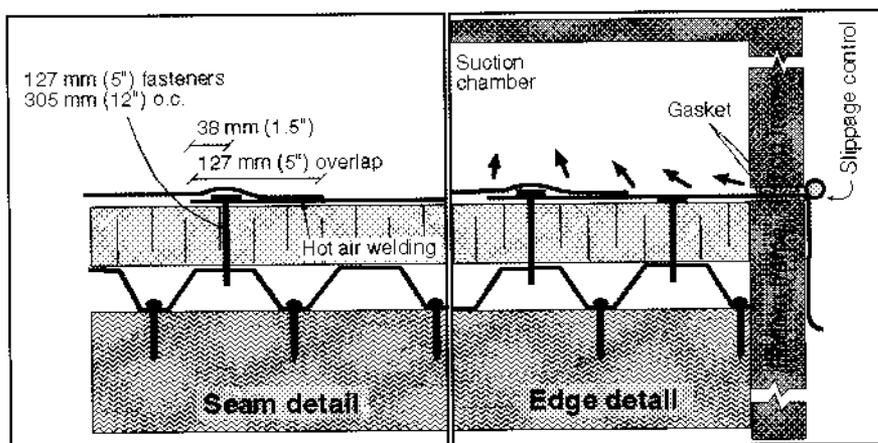
**Figure 2: TPO System Layout with seam and edge detail**
