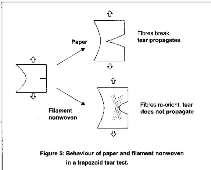
In **Figure 5** the tearing behaviour of paper and filament nonwoven are schematically represented and **Figure 5A** shows a few pictures taken during trapezoid tear tests.
