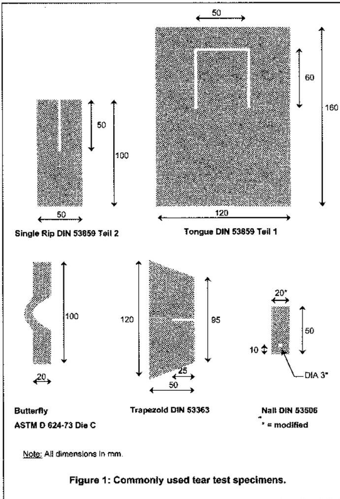
The single rip and tongue tear tests simulate the way one would tear up a piece of paper or nonwoven. As they are among the most commonly used tests they have been employed in this study.
